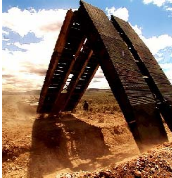
Figure 1 AVLB in the launching position
