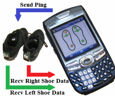
Fig. 4. The smartphone and shoes communication routine over Bluetooth.
